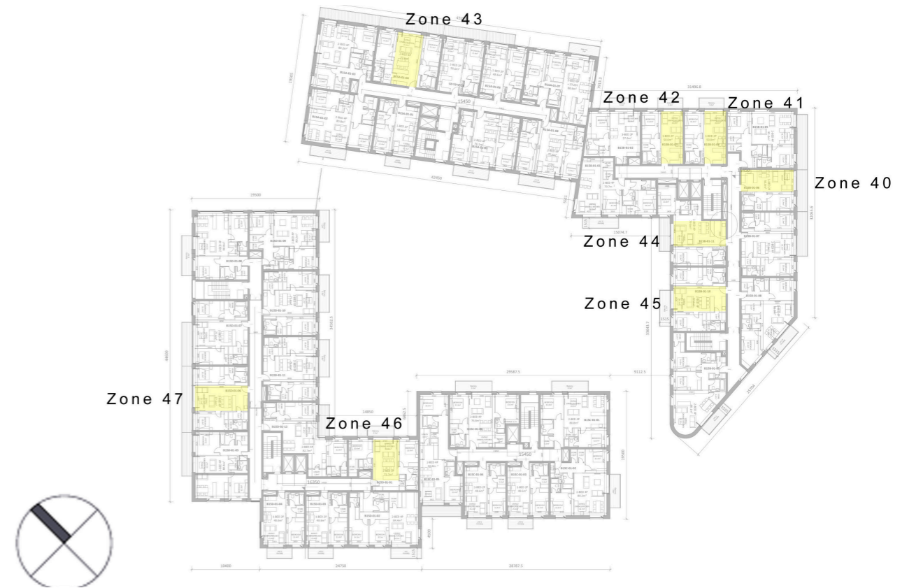
Figure 5.10: Indicative diagram based on floor plan prepared by O'Mahony Pike Architects showing location of sample rooms (in yellow) analysed as part of this assessment of daylight access within the proposed development – annotated in yellow by ARC - Block 15 - Floor 01
