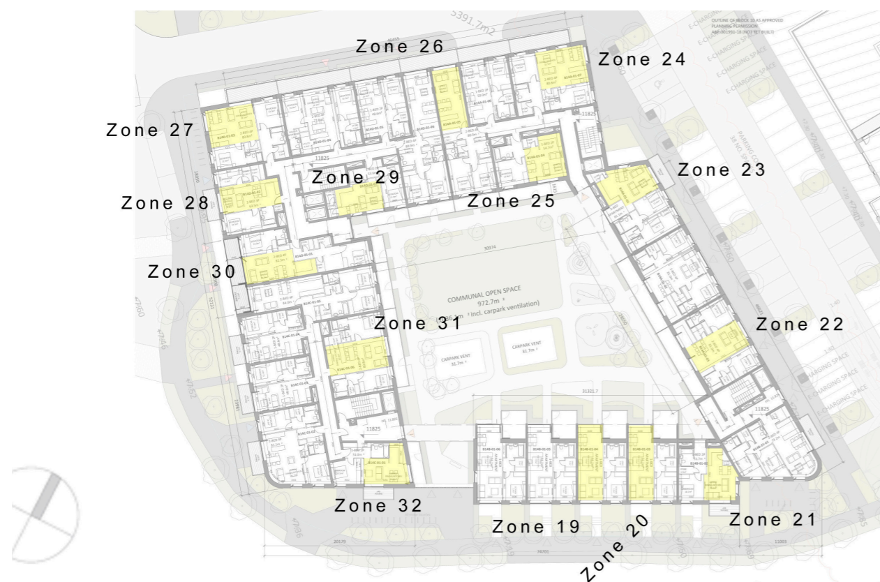
Figure 5.6: Indicative diagram based on floor plan prepared by O'Mahony Pike Architects showing location of sample rooms (in yellow) analysed as part of this assessment of daylight access within the proposed development – annotated in yellow by ARC - Block 14 - Floor 01
