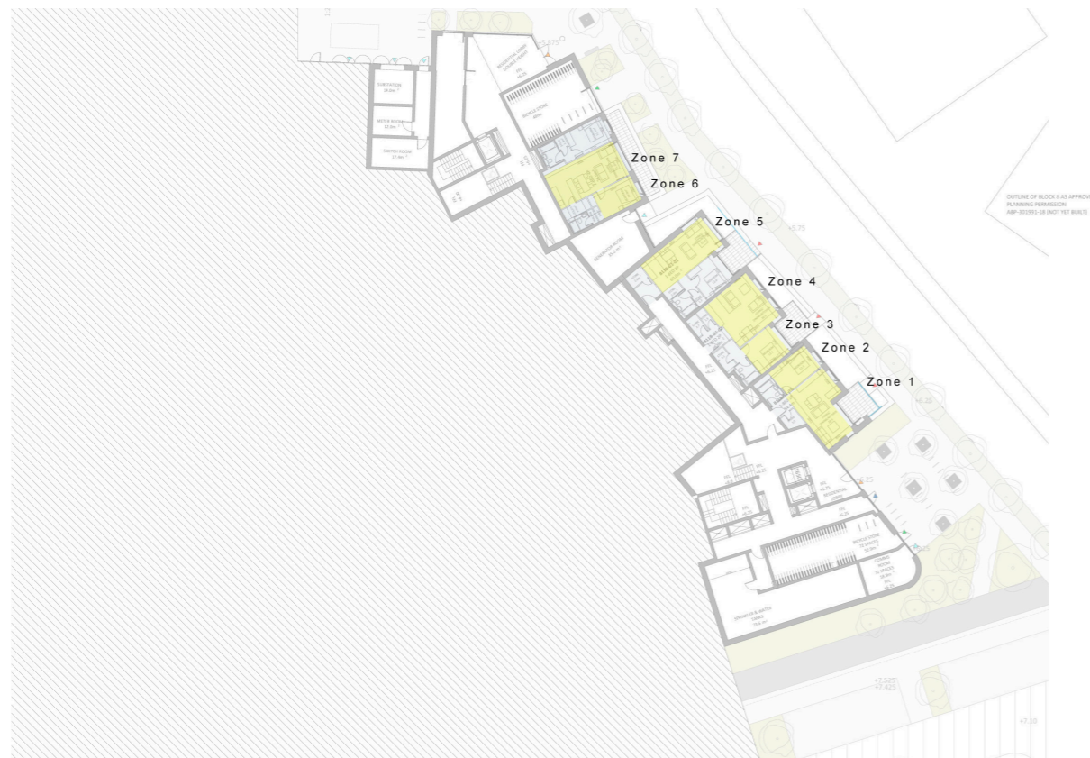
Figure 5.1: Indicative diagram based on floor plan prepared by O'Mahony Pike Architects showing location of sample rooms (in yellow) analysed as part of this assessment of daylight access within the proposed development – annotated in yellow by ARC - Block 11 - Floor G1
