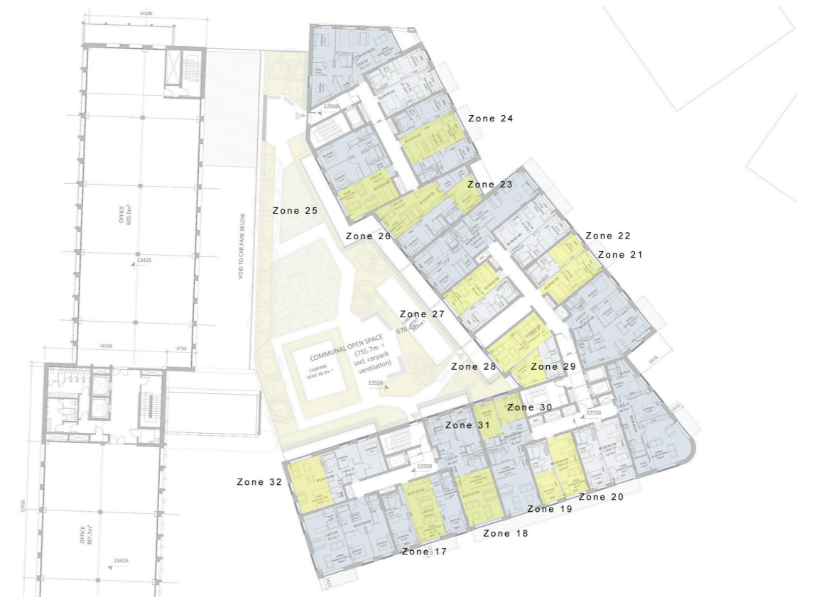
Figure 5.3: Indicative diagram based on floor plan prepared by O'Mahony Pike Architects showing location of sample rooms (in yellow) analysed as part of this assessment of daylight access within the proposed development – annotated in yellow by ARC - Block 11 - Floor 01
