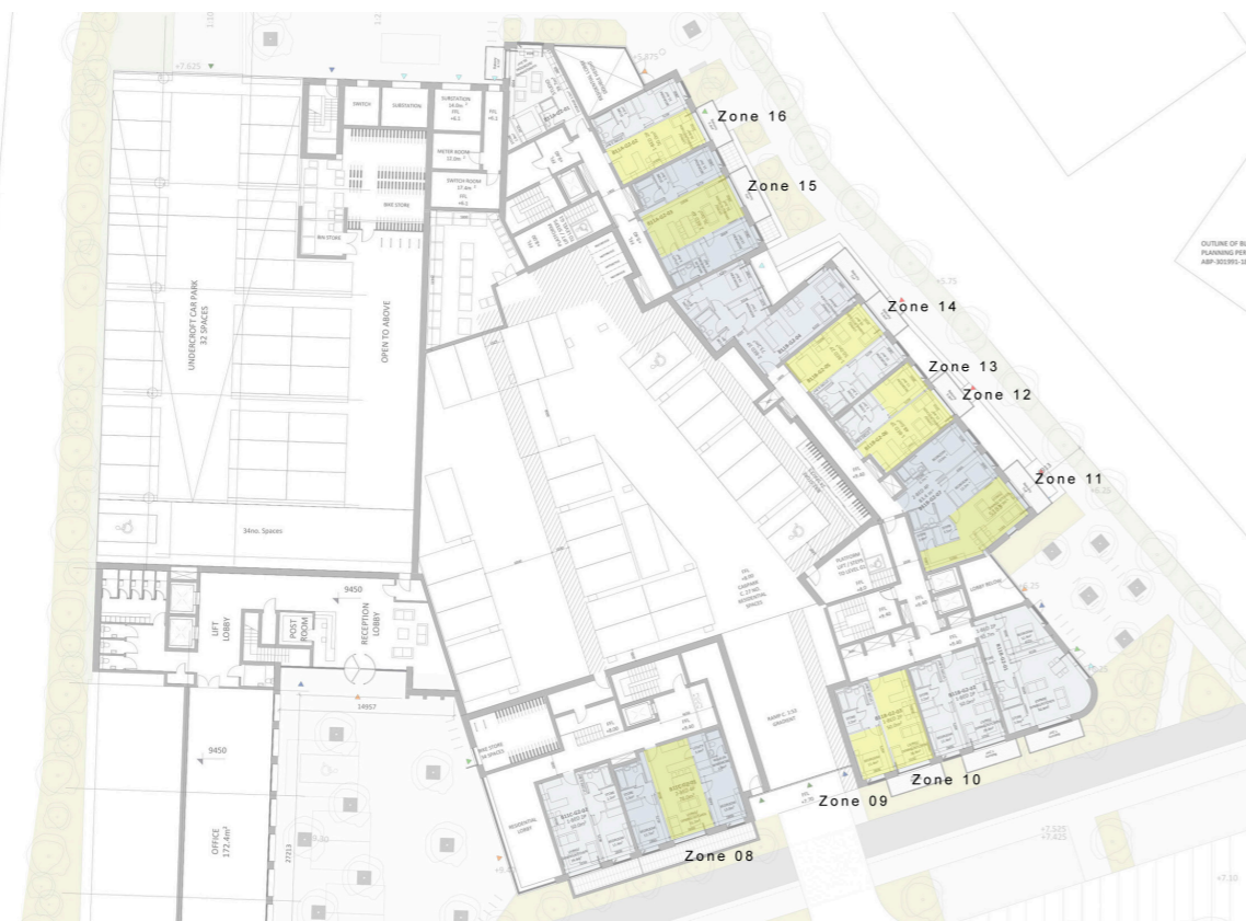
Figure 5.2: Indicative diagram based on floor plan prepared by O'Mahony Pike Architects showing location of sample rooms (in yellow) analysed as part of this assessment of daylight access within the proposed development – annotated in yellow by ARC - Block 11 - Floor G2
