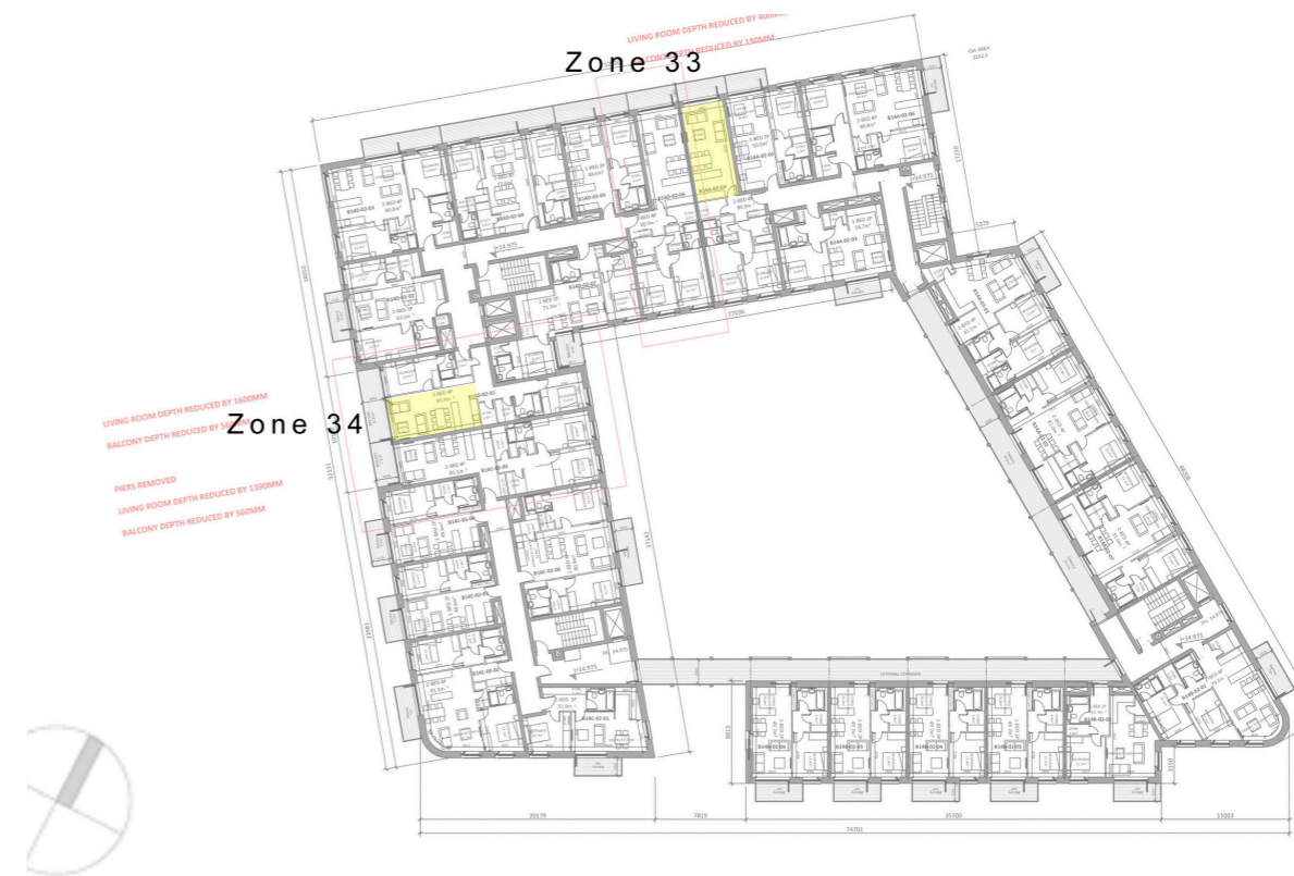
Figure 5.7: Indicative diagram based on floor plan prepared by O'Mahony Pike Architects showing location of sample rooms (in yellow) analysed as part of this assessment of daylight access within the proposed development – annotated in yellow by ARC - Block 14 - Floor 02
