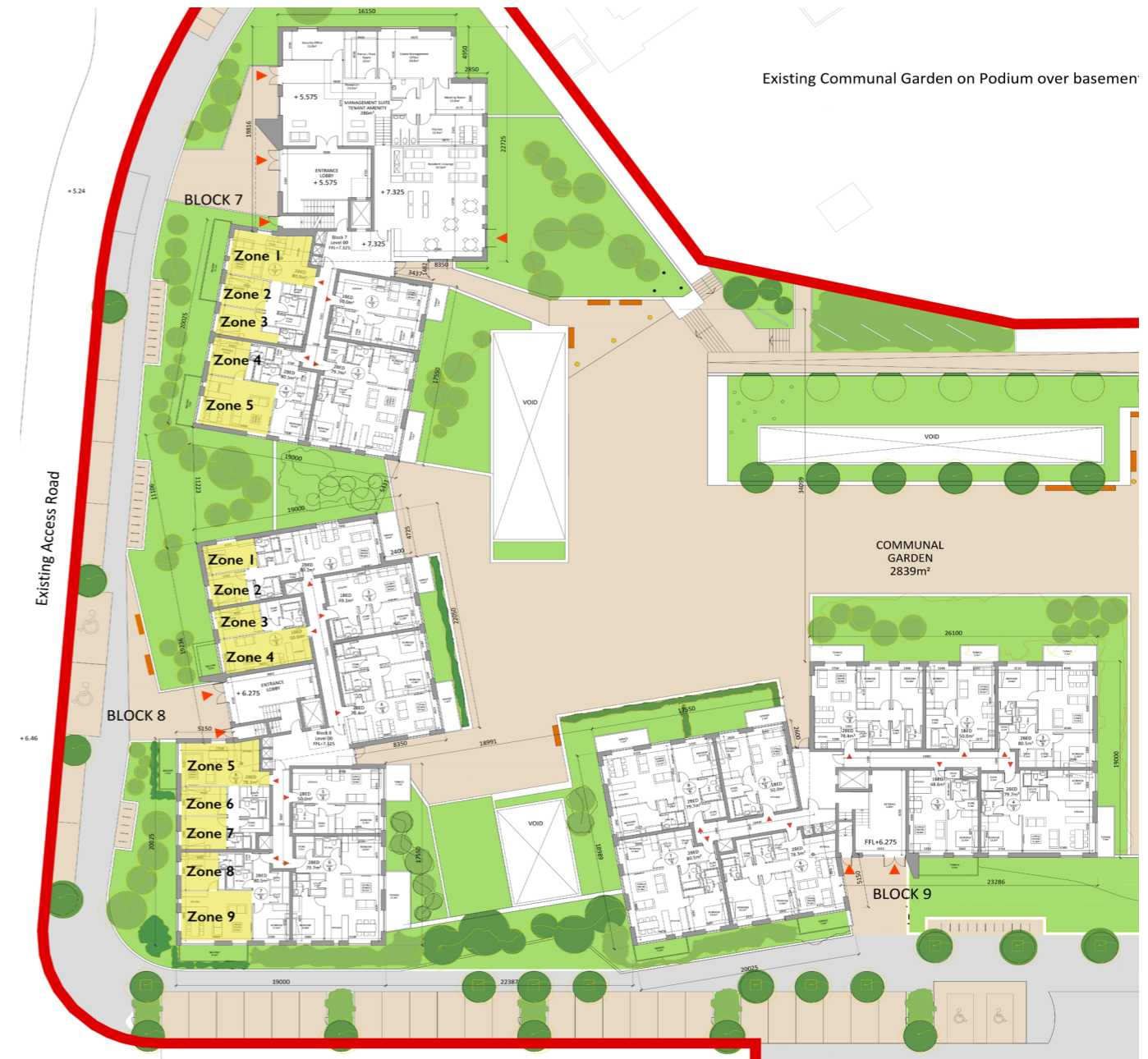
Figure 3.5: Indicative diagram based on floor plan prepared by O'Mahony Pike Architects showing location of sample rooms (in yellow) analysed as part of this assessment of daylight access within the proposed development – annotated in yellow by ARC - Blocks 7 and 8 - Floor 00
